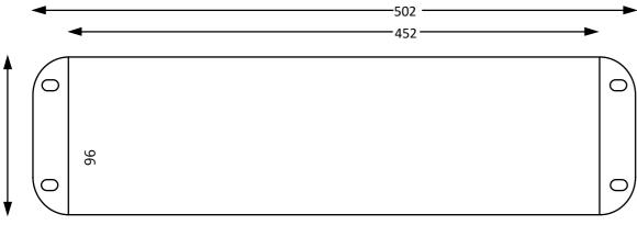
Fixing Holes M6 Product Height 60mm All Dimensions in mm Drawing not to Scale
